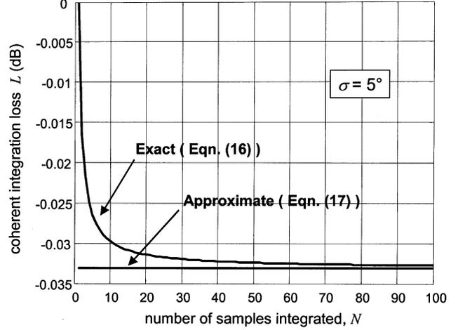
Fig. 1. Comparison of “exact” formula for the change in integrated power due to phase noise (16) to the simplified approximation (17) as a function of the number of samples integrated  $N$ .  $\sigma = 5^\circ$ .
