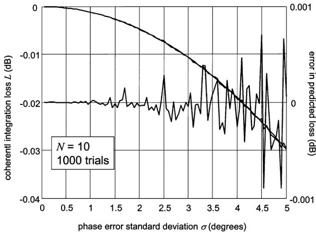
Fig. 2. Agreement between simulated and analytically estimated (16) coherent integration loss due to phase noise.  $N = 10$  samples integrated, 1000 Monte Carlo trials. (Left ordinate) Simulated and predicted integration loss are nearly indistinguishable. (Right ordinate) Difference in the two curves. For this case, it is well under 0.001 dB.
