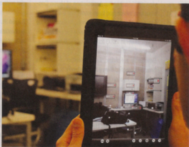
'INFOSPOTTING' Georgia Tech student researcher Ebrahim Karan pulls up BIM data using an iPad camera loaded with the InfoSPOT prototype.
